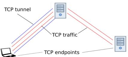
This is implemented using special IP packets which carry the traffic to the receiver within an IP packet sent to the "relay" point.
